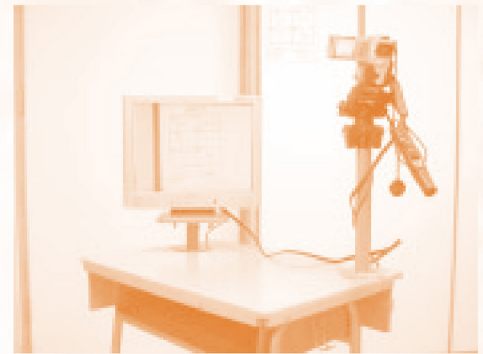
遠近佳儀 Digicam-Monitor-Magnifier Compact Visual System for Low-vision Students
